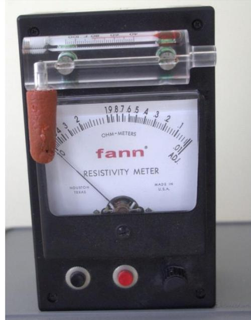
**Device: Model 653B Resistivity Meter**
