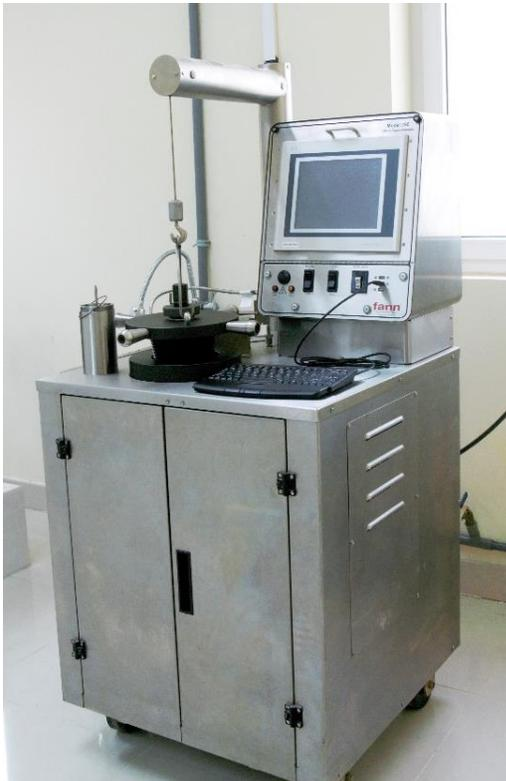
**Device: HPHT Consistometer Model 290**
