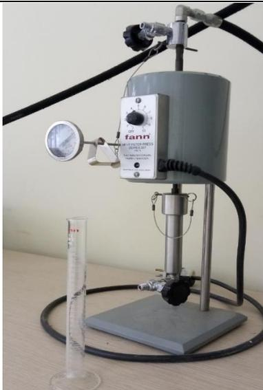
**Device: HPHT Filter Presses**
