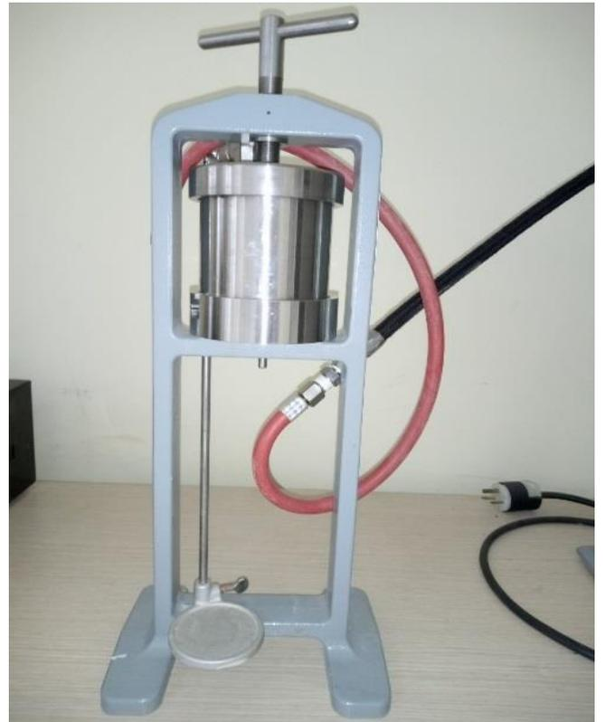
**Device: Low Temperature (LPLT) Filter Presses**
