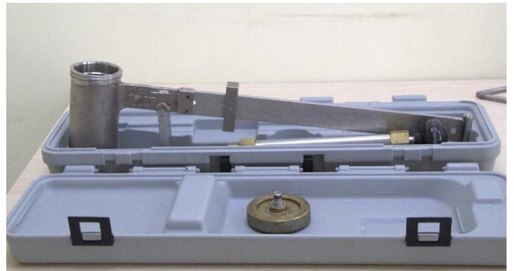
**Device: Balance Density TruWate Model 141**
