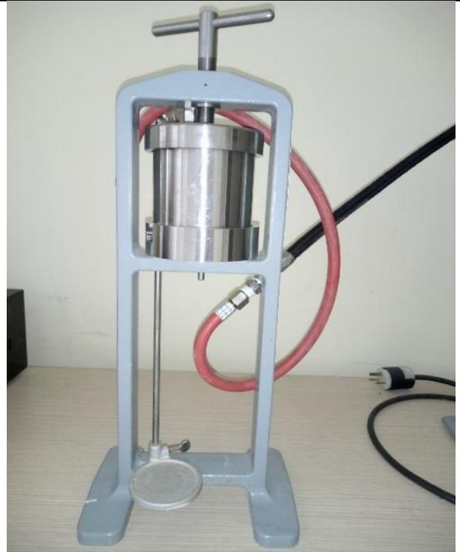
**Device: Low Temperature (LPLT) Filter Presses**
