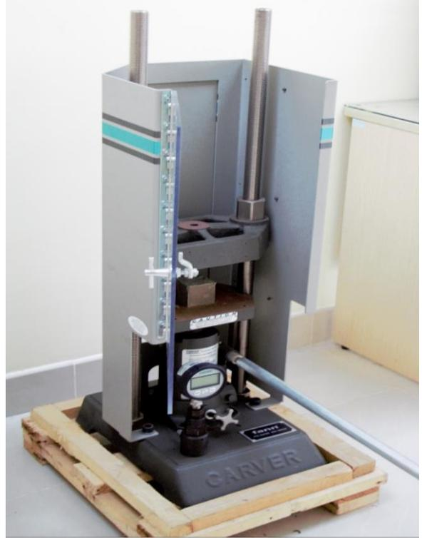
**Device: Compressive Strength Tester**
