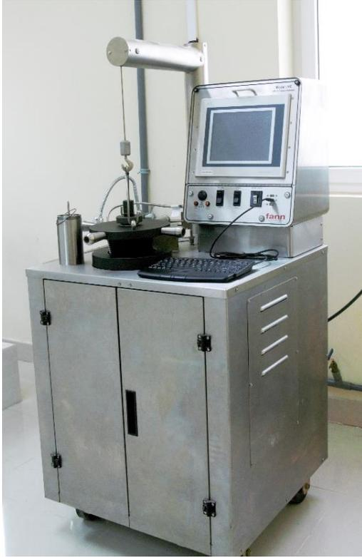
**Device: HPHT Consistometer Model 290**
