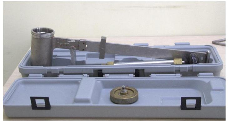
**Device: Balance Density TruWate Model 141**
