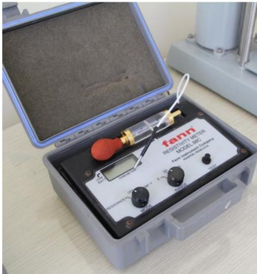
**Device: Resistivity Meter Model 88C**
