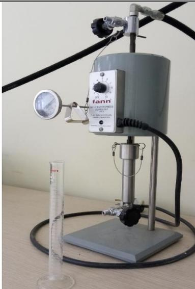
**Device: HPHT Filter Presses**
