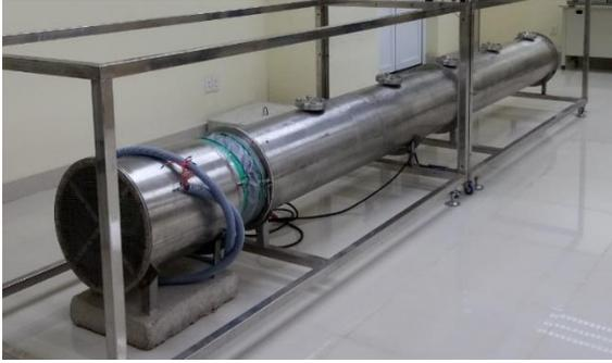
**Device: Velocity distribution of flowing fluid in pipe**
